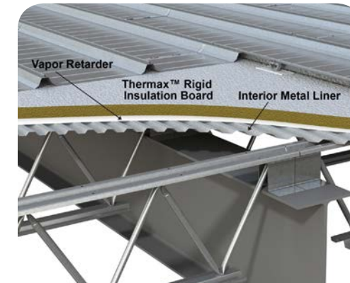
The CMR-24 roof system adds a layer of rigid insulation board and an interior liner to the MR-24 roof system for superior energy efficiency.
